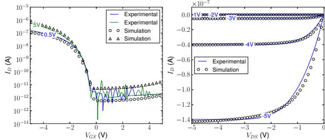
Fig. 3: Comparison of measured and modeled static output and transfer characteristics of an OTFT
