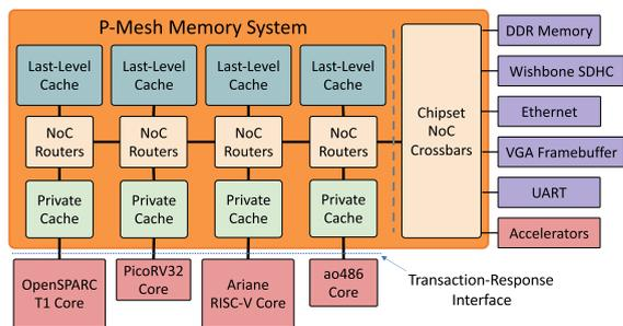
**Figure 2.** OpenPiton architecture, adapted.<sup>1</sup>
