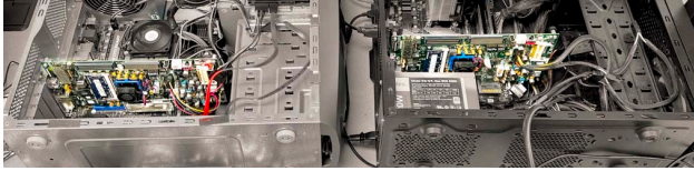
Figure 5: Evaluation platform including FPGA boards which the customized memory controller is programmed on.
